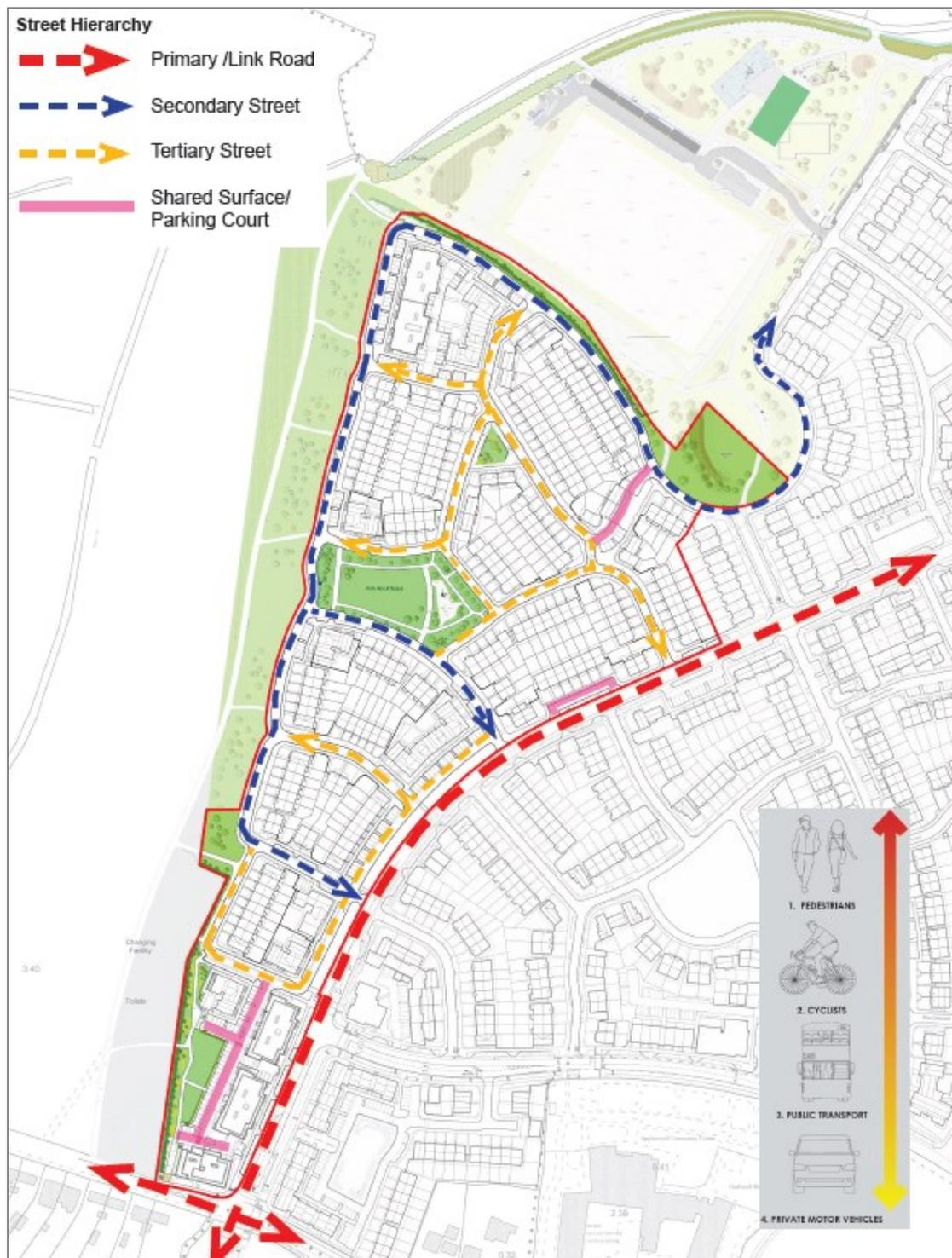
Figure 1. Proposed Connection within the Hierarchy of Street Network in the Scheme
